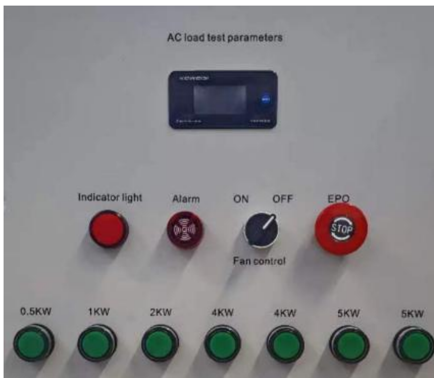
AC voltage and current power meter: Display the single-item voltage and current power
